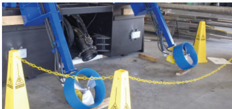
Dual prop drive self-propulsion system
