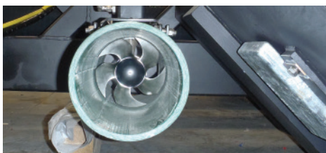
Bow thruster for side current correction & quick turns.
