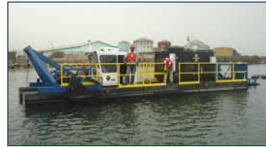
A Model 7012 HP Versi-Dredge® mines sand from a river in Monrovia, Liberia.
