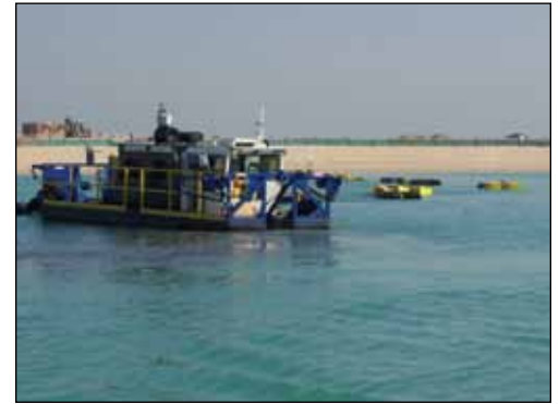
A Model 5012 LP removes silt from channels at a resort in the Middle East.
