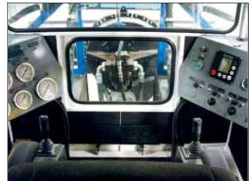
All Versi-Dredge® models come standard with joystick controls and oversized gauges for ease of operation.
