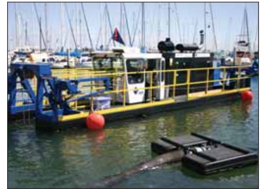
A Model 5012 HP removes sand from a large marina in California.
